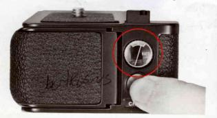
side of battery pack and watch the indicator needle. If it swings into the green region or beyond, the batteries are still good. If not, replace all the batteries.
